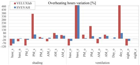
Figure 2. Variation of overheating hours in percentage, calculated according to AH Specifications, 2<sup>nd</sup> edition (2013) (www.activehouse.info) and compared to baseline scenario.
