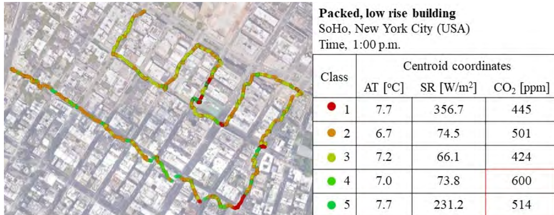
Figure 3. Spatial distribution of the five data clusters (k=5) obtained in SoHo, New York City.
