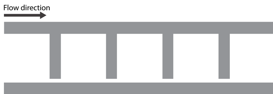
Fig. 3. Schematic of labyrinth seal 2 calculation domain
