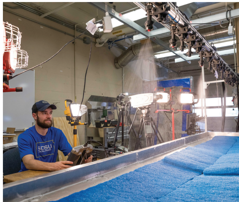
Ryan Fouts, a senior mechanical engineering major at South Dakota State University, captures high-speed video of the nozzles on the sprayer test bed he helped build in summer 2019.
