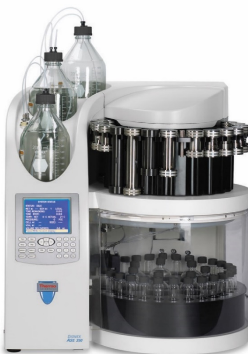
Figure 2.2 Image of Dionex™ ASE™ 350 Accelerated Solvent Extractor used in this research work. (Image obtained from ThermoFisher Scientific).
