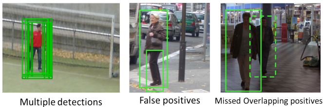
Fig. 6. Difficulties that non-maximum suppression tackles. Detections are in green. Best viewed in color.
