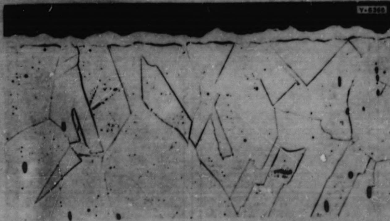
Fig. 61. Section of an As-Tested Type-316 Stainless Steel 0.505-in. Tensile Test Bar Brazed with a 60% Pd-37% Ni-3% Si Alloy. The bar fractured in a brittle manner at 48,500 psi, and the elongation in a 2-in.-gage length was 7%. Fracture occurred along the center of the brazed joint. Etched with aqua regia. 200X.
