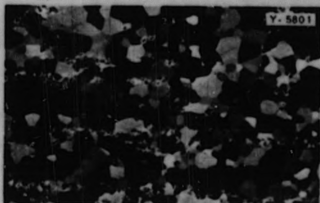
(b) 9/10-in.-dia extruded rod; middle of extruded length (U10-X5)
