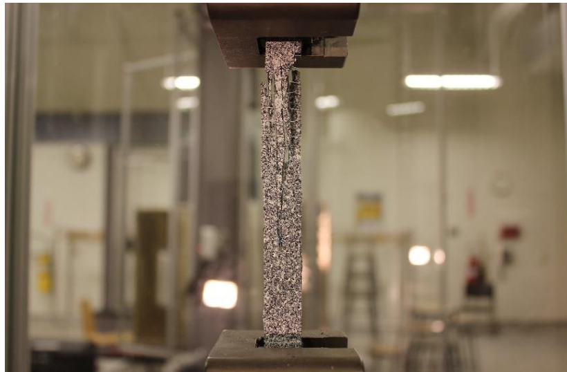
Figure 3.14: Basalt coupon under uniaxial tension test
