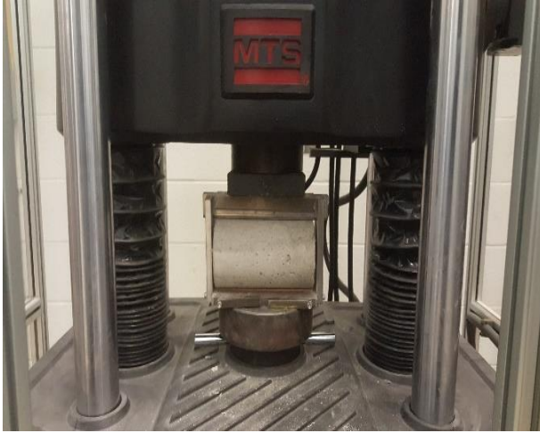
Figure 3.6: Split tensile test
