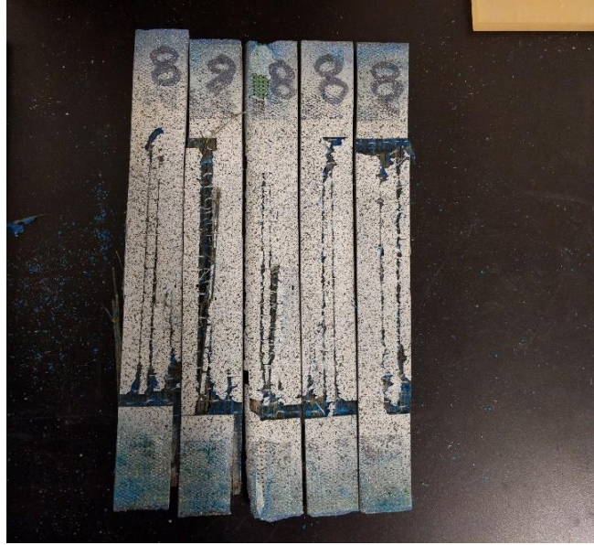
Figure 3.15: Basalt coupons after uniaxial testing
