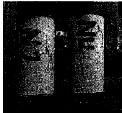
Figure 3.14 Failed grout cylinders
