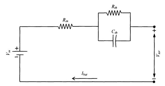
Fig. 3.6: Thevenin electric circuit model.
