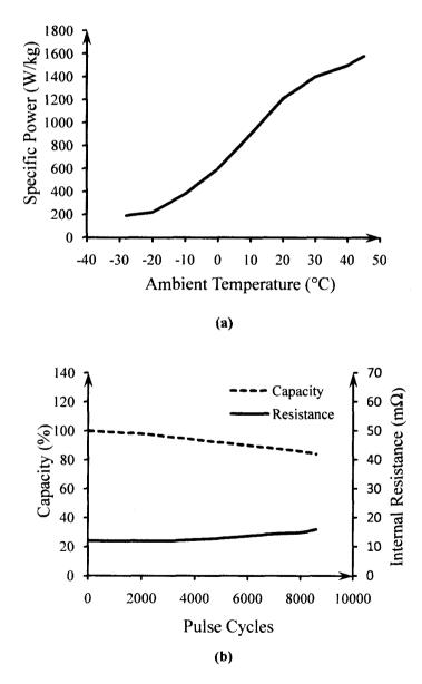
Fig. 2.6: Performance characteristics of Panasonic NiMH module. (a) Specific power for varying operating temperature. (b) Change in internal resistance over the cycle life.
