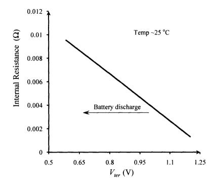
Fig. 3.15: Battery terminal voltage ( $V_{ter}$ ) as a function of internal resistance.
