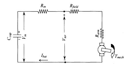
Fig. 4.13: Electric drivetrain model using DC series motor.
