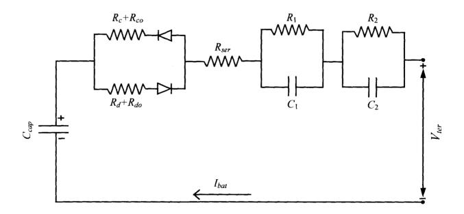
Fig. 3.10: Capacitive representation of the battery model.
