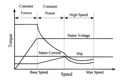
Fig. 4.7: Induction motor operation characteristics.
