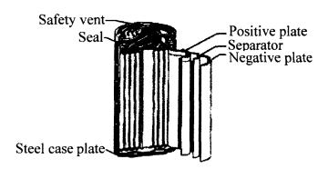
Fig. 2.5: NiMH Cylindrical battery construction.
