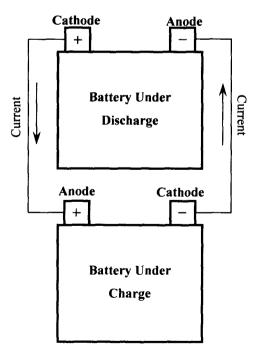
Fig. 2.2: Battery charge-discharge operation.
