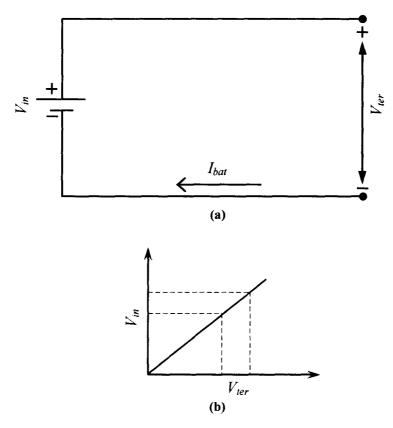
Fig. 3.3: (a) Ideal electric circuit model (b) Battery terminal voltage  $(V_{ter})$  as a function of internal generated voltage  $(V_{in})$ .
