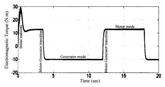
Fig. 4. 17: Electromagnetic torque analysis of DC motor.
