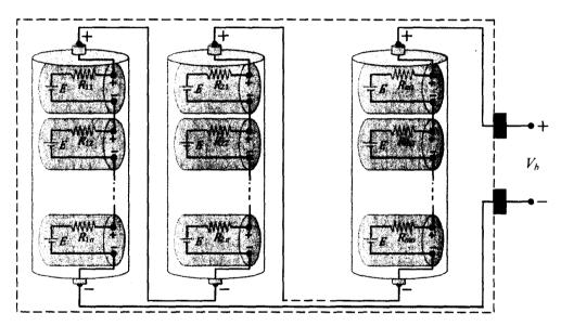
Fig. 4.2: Schematic representation of the battery pack.
