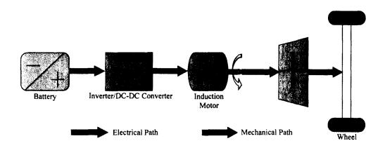
Fig. 4.14: Electric drivetrain using induction motor.
