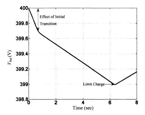
Fig. 4. 22: Battery charge-discharge characteristics across induction motor.
