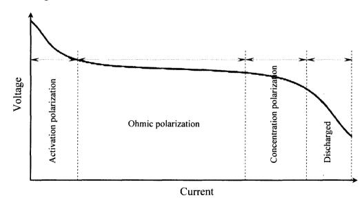
Fig. 3.2: Voltage-current behavior of electrochemical cells.
