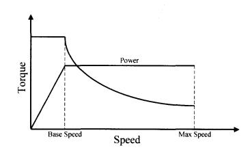
Fig. 4.4: HEV/EV traction motor requisites.
