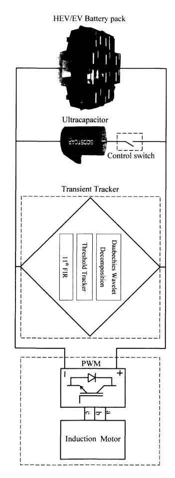
Fig. 5.6: Parallel battery and ultracapacitor operation.
