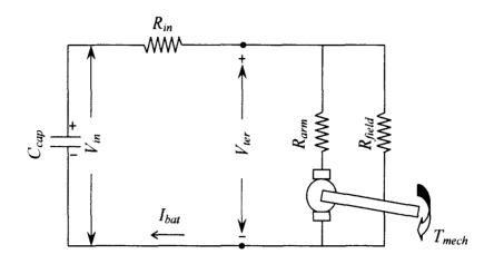
Fig. 4.12: Electric drivetrain model using DC shunt motor.
