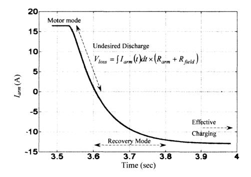
Fig. 4. 19: Result of torque on the battery charge-discharge current.
