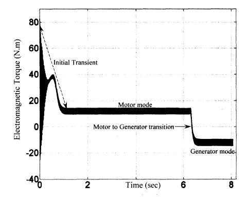
Fig. 4. 21: Electromagnetic torque of induction motor.
