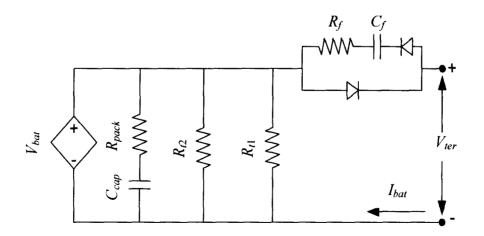
Fig. 4.10: Battery pack model.
