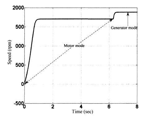
Fig. 4. 23: Induction motor speed variation for motor and generator mode.
