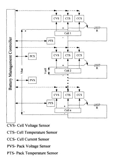
Fig. 4.3: Schematic representation of the battery management system.
