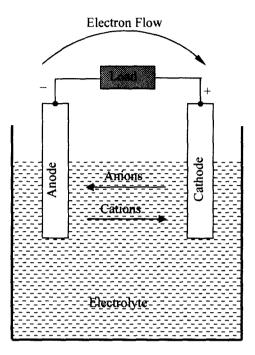
Fig. 2.1: Electrochemical reaction in a cell during discharge.
