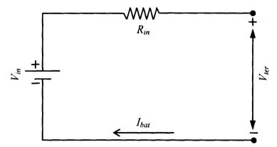
Fig. 3.4: Linear electric circuit model.
