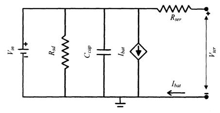
Fig. 3.8: Runtime based model.
