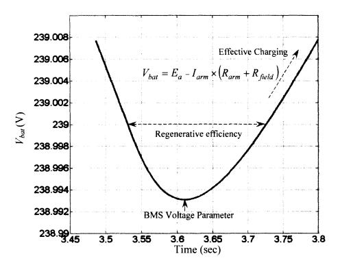
Fig. 4. 20: Location of BMS voltage parameter for DC motor.
