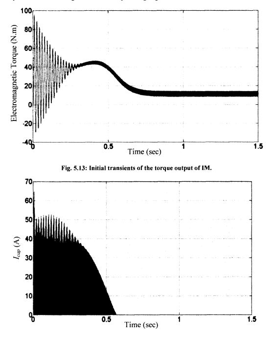
Fig. 5.14: Ultracapacitor current variation in accordance with the torque production.
