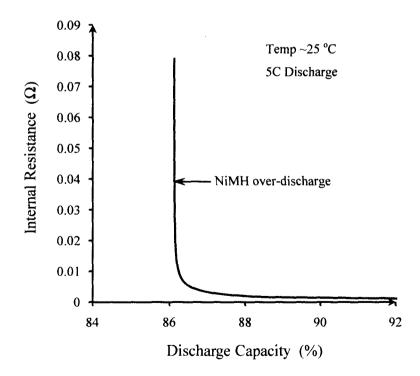
Fig.3.16: Internal resistance drop as a function of SOC.
