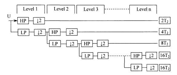
Fig. 5.2: n-level asymmetric filter bank analysis.
