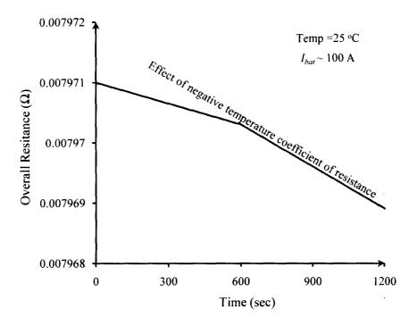
Fig.3.21: The change in resistance as a function of time.
