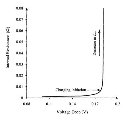
Fig.3.18: Voltage drop with respect to internal resistance.
