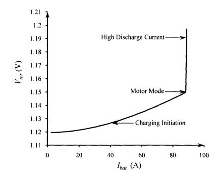
Fig.3.17: Battery terminal voltage ( $V_{ter}$ ) as a function of battery current ( $I_{bat}$ ).
