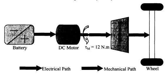
Fig. 4.11: Electric drivetrain using DC motor.
