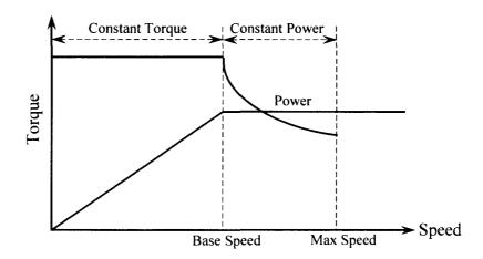
Fig. 4.9: Permanent magnet synchronous motor operation characteristics.
