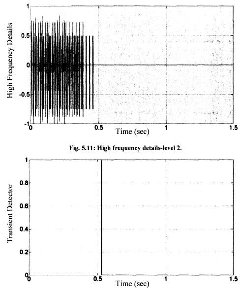
Fig. 5.12: Transient detector output.
