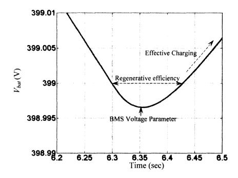
Fig. 4. 24: Motor-generator transition mode analysis for induction motor.
