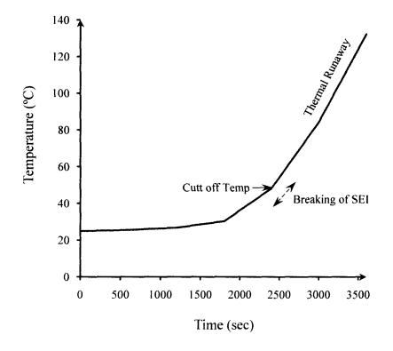
Fig.3.24: Temperature profile across the complete simulation.
