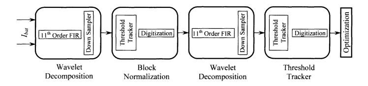
Fig. 5.1: Transient detection using wavelet decomposition.
