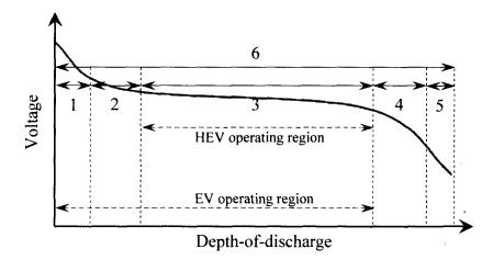
Fig. 3.11: Battery model illustration.
