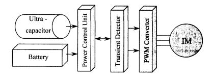
Fig. 5.5: Energy storage control architecture.
