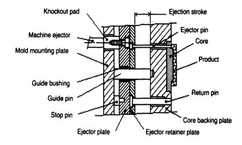
Figure 5.6: Typical mould with ejector pins [38]
