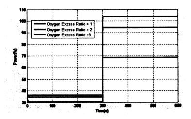
Figure 27. Fuel cell power response in different oxygen excess ratio
