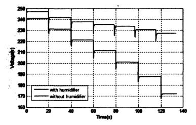
Figure 15. Output voltages with and without humidifier control
