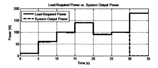
Figure 35. Load-Required Power vs. System Produced Power
