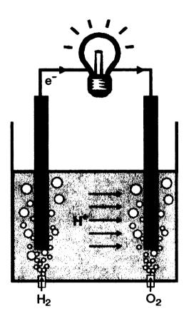
Figure 1. A Simple fuel cell operation[1]
