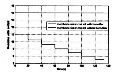
Figure 18. Membrane water content with and without humidifier control
