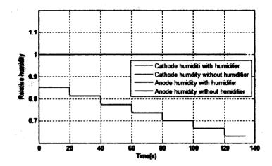
Figure 17. Relative humidity with and without humidifier control
