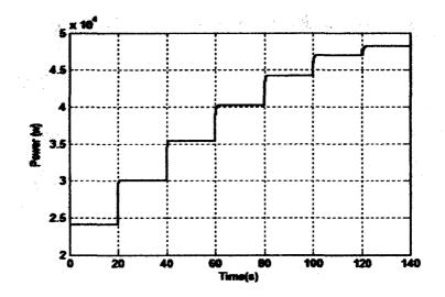
Figure 11. PEM fuel cell output power response
