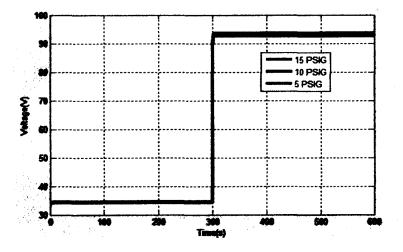
Figure 25. Fuel cell power response in different cathode inlet pressure
