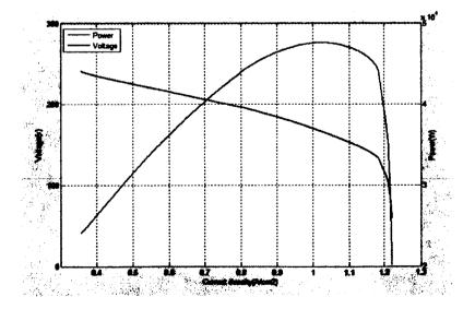
Figure 7. PEM fuel cell polarization characteristic
