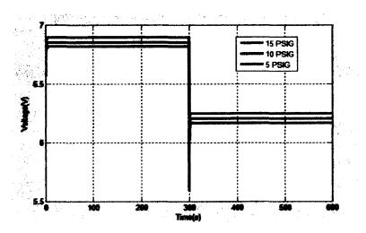
Figure 24. Fuel cell voltage response in different cathode inlet pressure
