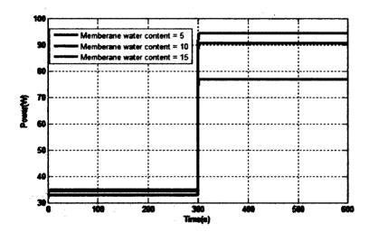
Figure 23. Fuel cell power response in different membrane water content
