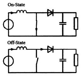
Figure 4. On-off state explained of boost DC/DC converter
