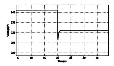
Figure 10. Output voltage transient when input current change from 100A to 130A
