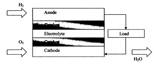
Figure 2. PEM fuel cell operation
