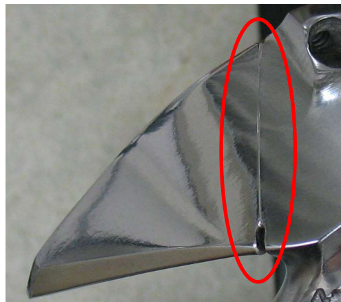
Fig. 2 - Wear damage caused by the thread on a used bobbin case
