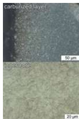
248 Fig. 3 Structural features of the carburized layer and of the inner core of the AISI 5115 samples, after the 249 heat treatment sequence
