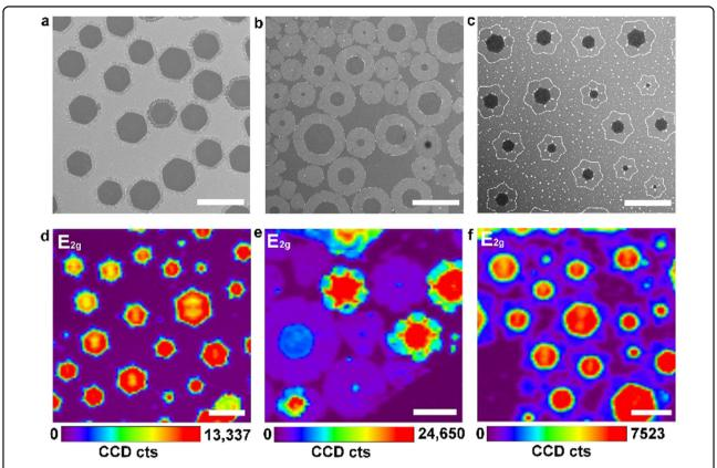
Fig. 2 Shape engineering of G-h-BN flakes on a liquid Cu surface. a Hexagonal G-h-BN flake. b Concave-shaped G-h-BN flake. c Flower-like G-h-BN flake. d-f Raman mapping images of the corresponding three shaped flakes for the  $E_{2q}$  peak at 1371 cm<sup>-1</sup>. All scale bars are 10  $\mu$ m
