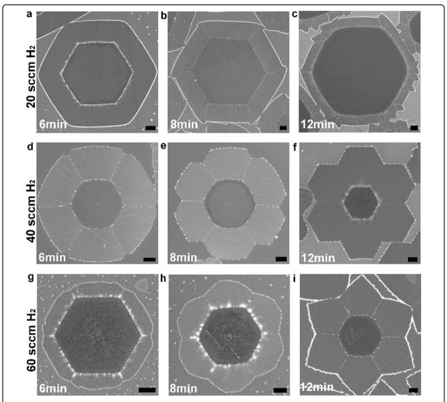
Fig. 3 The shape evolution of the three kinds G-h-BN flakes. a–c Shape evolution of hexagonal G-h-BN flake. d–f Shape evolution of concave G-h-BN flakes. g–i Shape evolution of flower-like G-h-BN flakes. All scale bars are 1 μm
