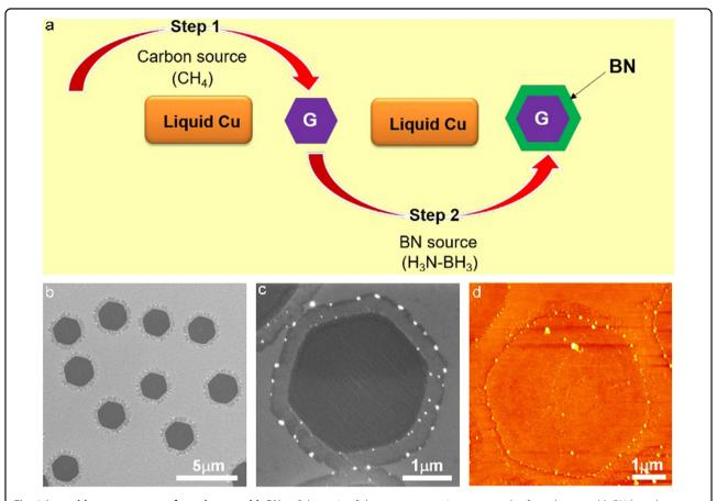
**Fig. 1 Lateral heterostructure of graphene and h-BN. a** Schematic of the two-step continuous growth of graphene and h-BN lateral heterostructure by CVD on a liquid Cu surface. **b, c** SEM images of large-area and single G-h-BN structures, respectively. Note that the subsequently grown h-BN has an epistrip morphology. **d** AFM image of a single G-h-BN flake
