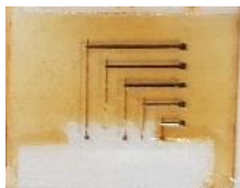
Attachment G- Burned PVP film caused by a lengthy treatment under an IR lamp.
