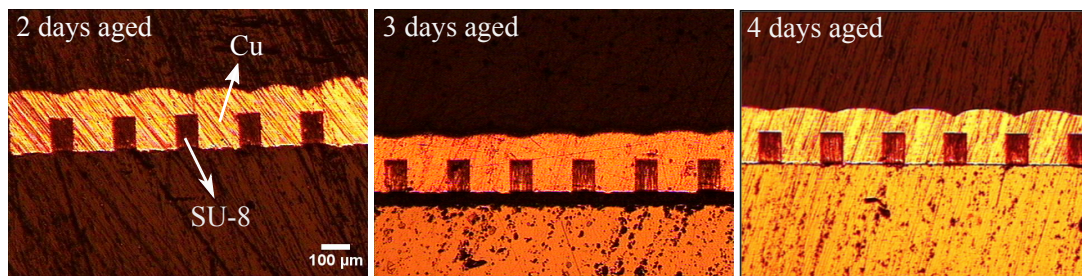
Figure 2.25. Cross-section of MMIs that electrodeposited in aged electrolyte.
