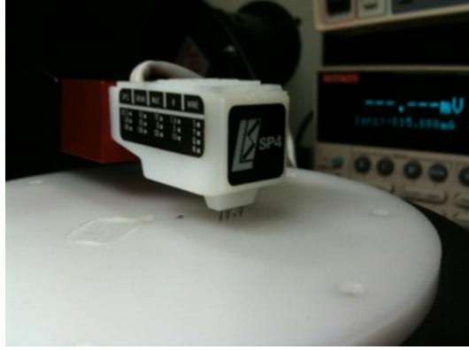
Figure 2.5. Setup of four-point probe device.
