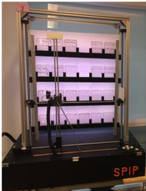
Supp. Fig. 15 SPIP 1 featured two axis movement, IR range finders, and manual control through push button controls. Image taken at Life Sciences Week, 2016
