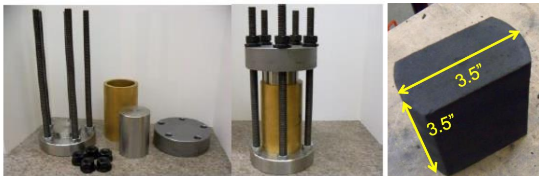
Figure 8. The die used in the production of monoliths. Left: The die assembly. Right: An example of one of the finished monoliths that was machined to use in a different tank in our lab.
