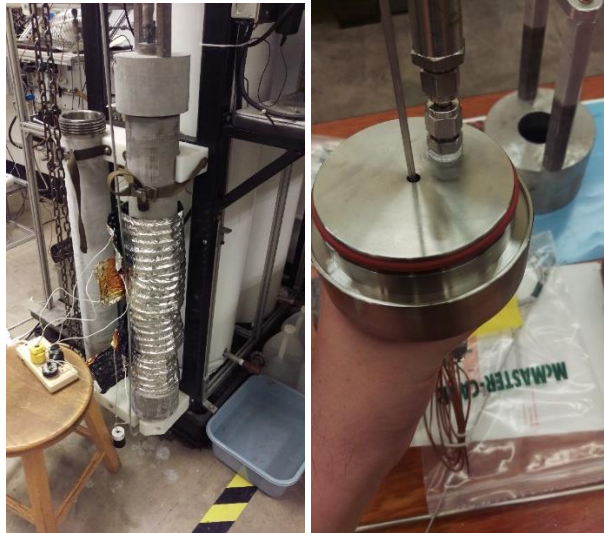
Figure 15. Tank being outgassed with heating jackets and top end cap with silicone O-ring around the shaft groove and no O-ring on the face seal.
