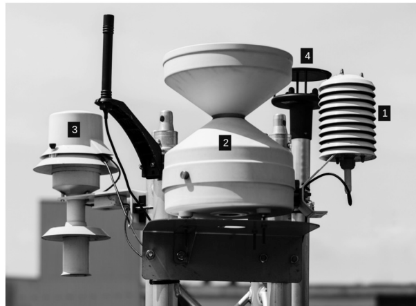
Fig. 2. Sensors of a MOCCA weather station: (1) passively ventilated radiation shield containing a temperature and relative humidity sensor, (2) rain gauge, (3) actively ventilated radiation shield containing a temperature sensor and (4) ultrasonic anemometer.
