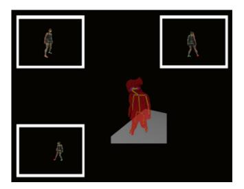
By combining 2D-camera input, a full 3D-reconstruction (middle) including joint recognition is created.
