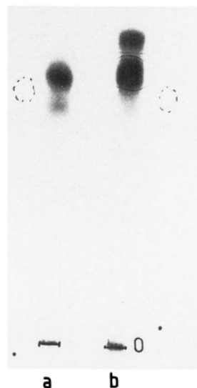
FIG. 4. Electrophoresis of the tubulin synthetic peptide phosphorylated in vitro by casein kinase II. The synthetic peptide EMYEDDEEESQGPK was phosphorylated in vitro with casein kinase II as indicated under "Experimental Procedures," in the presence of 0.1 mM ATP. The phosphopeptide was further incubated in the absence (a) or presence (b) of S. aureus V8 protease and the labeled peptides subjected to thin layer electrophoresis in pH 6.3 buffer (10% pyridine, 0.5% acetic acid), followed by autoradiography, that is shown in the figure. To trace the electrophoretic mobility from the origin (O), orange G was used. The electrophoresis was stopped when the marker reached the position indicated by the circled discontinuous line. The major spot marked in lane a corresponds to the phosphorylated synthetic peptide. The minor spot with a lower electrophoretic mobility which is also found in lane a corresponds to a peptide lacking the amino-terminal glutamate residue of the synthetic peptide as a consequence of a low yield in the last step of the synthesis procedure. The spots marked in lane b were subjected to gas-phase sequencing as indicated in the text.
