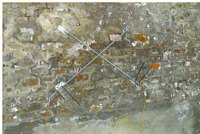
Figure 5: Arrange of the measurement system for recording shear forces
