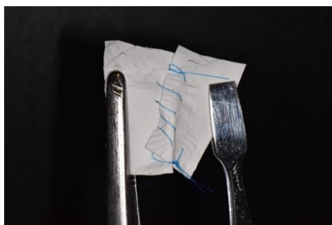
Figure 6. Nanofibre-based membrane obtained after 60 min of ELS with the following parameters: PCL 12% w/v in DCM/DMF 7:3, 17 kV potential, 27 G needle, 0.6 mL/h of flow rate. Nikon D3500, macro 105 Sigma tamron lens, Sigma ring flash. See the mechanical resistance during stretching the same membrane of Figure 5 after cut then sutured with 5/0 polypropylene.
