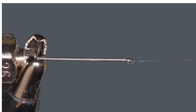
Figure 2. Taylor cone obtained with the following parameters: a solution of polycaprolactone (PCL) 12% w/v in dichloromethane/dimethylformamide (DCM/DMF) 7:3 applying 17 kV of potential and 0.6 mL/h of flow rate and using a 25 G needle. Nikon D3500, macro 105 Sigma tamron lens, Sigma ring flash.
