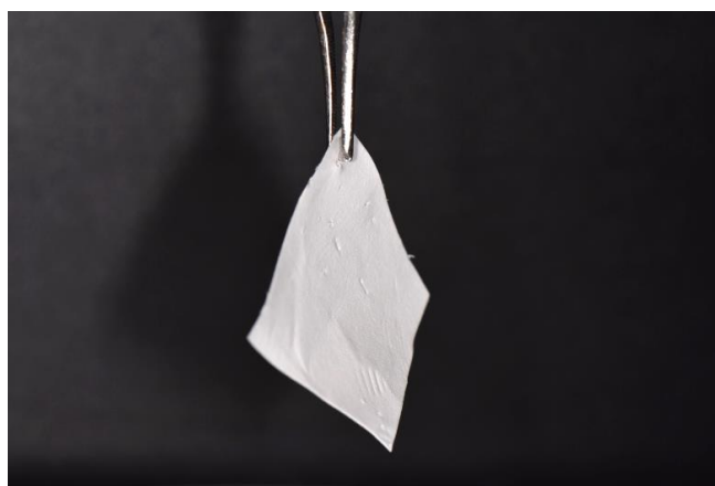
Figure 5. Nanofibre-based membrane obtained after 60 min of ELS with the following parameters: PCL 12% w/v in DCM/DMF 7:3, 17 kV potential, 27 G needle, 0.6 mL/h of flow rate. Nikon D3500, macro 105 Sigma tamron lens, Sigma ring flash. Membranes can be handled easily with surgical tweezers.
