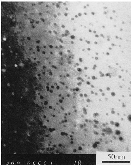
Fig. 13. Transmission electron micrograph of oxide particles in Mm13 cladding.
