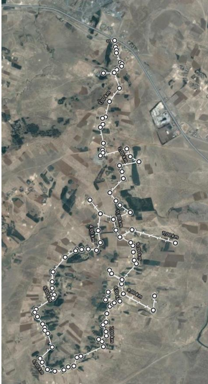
Figure 9. Satellite image of one of the 4 electrical grid extensions starting from the tarred road. Every dot resembles a household (courtyard) connection.
