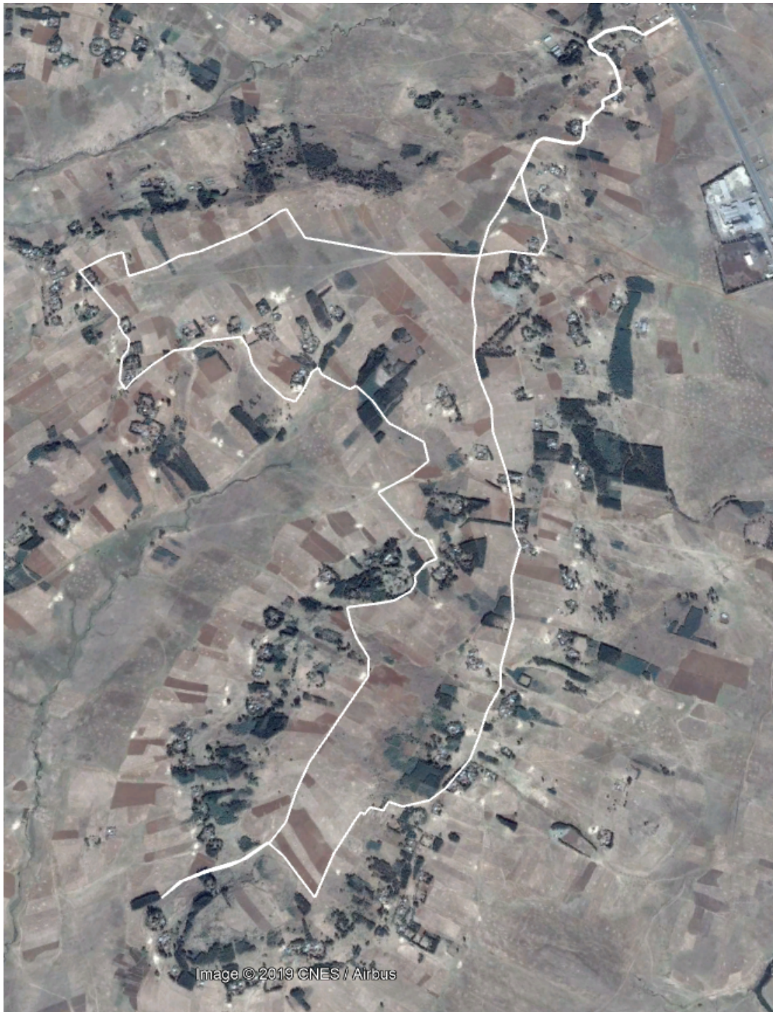
Figure 8 Satellite image of round 1 of the 3 possible milk collection rounds in the studied area to determine the driving distance. The selected route goes over single and double tracks. Rivers and steep slopes are avoided.
