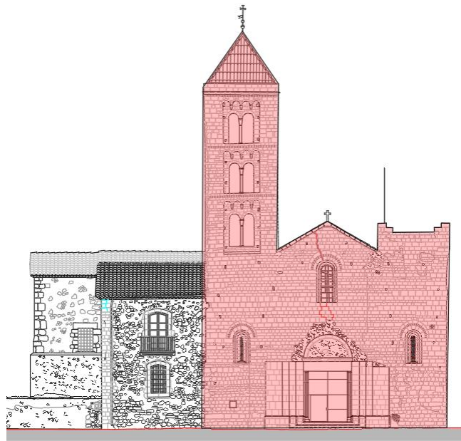
Figure 4.25. Overturning of the main façade of Vilabertran (V2)
