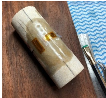
Figure 2-3 Core-plugs of Bentheimer sandstones drilled from quarried block and prepared by installation of strain gauges on the layer of epoxy resin at the centre point.
