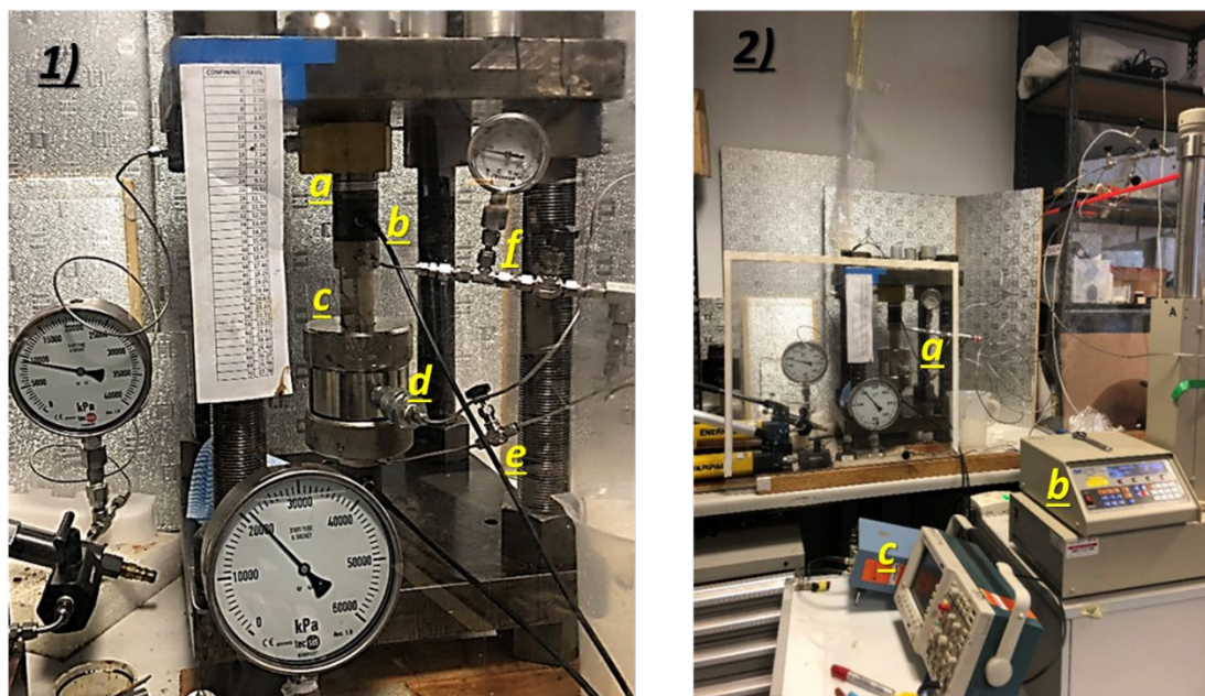
Figure 4-4 Layout of the experimental set-up: 1) Hook's cell and injection valves a) axial actuator, b) S-wave transducer, c) PEEK part, d) Hook's cell, e) input valve for fluid injection, and f) output valve for discharge and vacuum of the liquid. 2) a) hydrostatic pressure frame, b) pore pressure pump, and c) Ultrasonic bench equipment to record wavelets.
