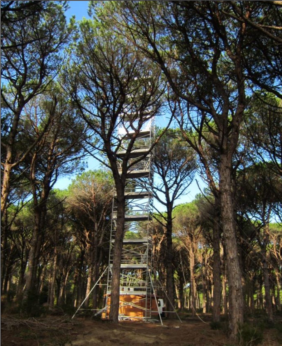
Fig. 56: the flux tower of 24 m at the Pinus pinea site in San Rossore
