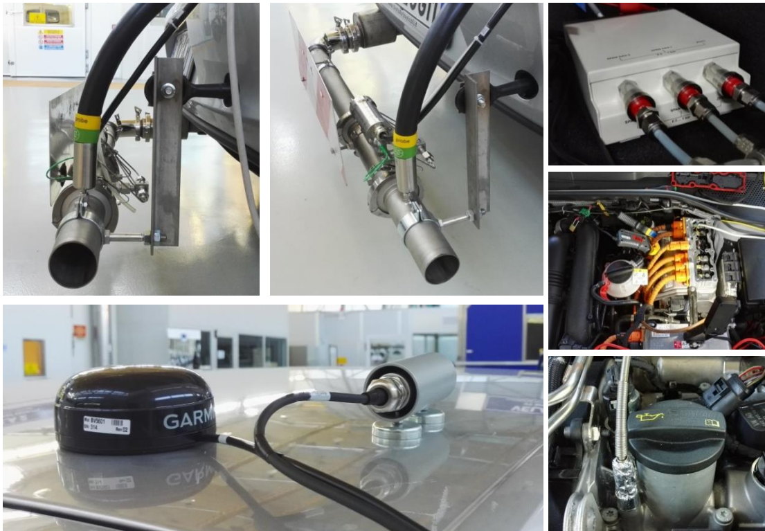
Figure 10: Positioning of GPS & weather station, of the flowmeter and of thermocouples.
