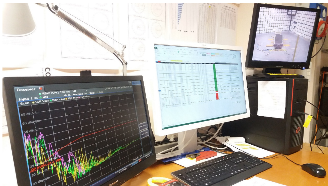
Figure 46: EMC tests monitoring, real-time trace analysis and data logging inside VeLA 9 control room
