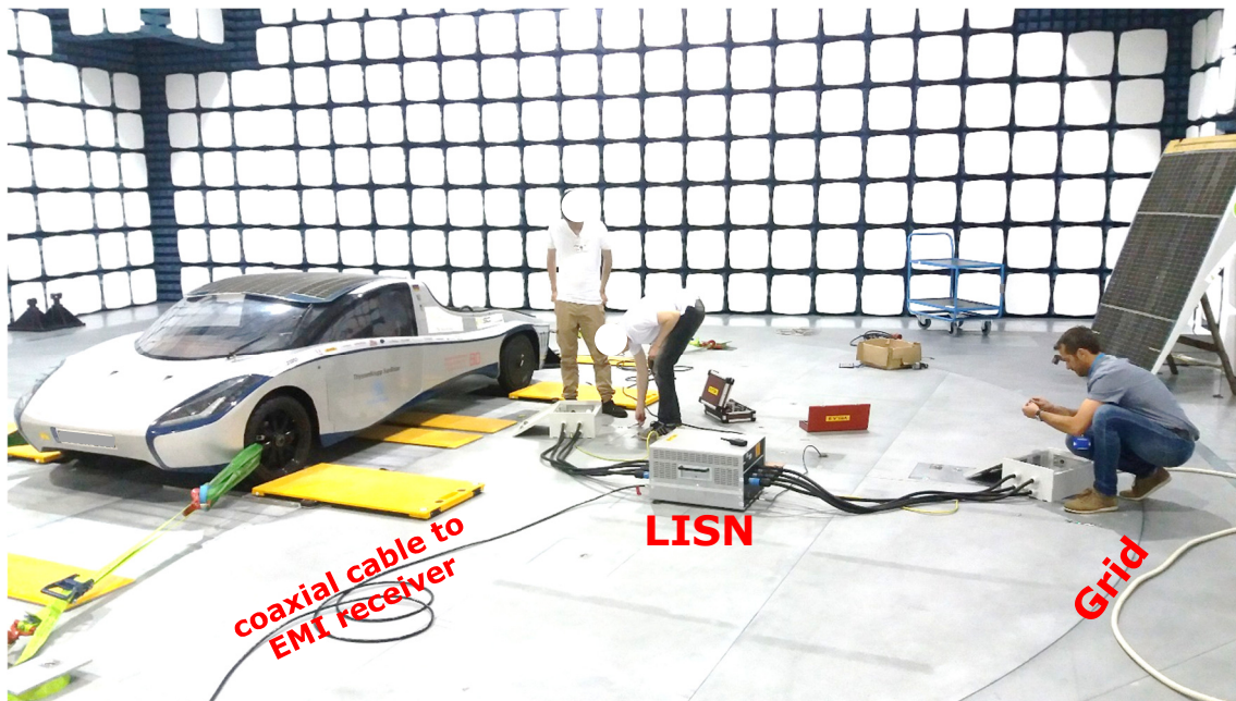
Figure 44: Setup and wire connections for testing the AC conducted emissions with a LISN during charging
