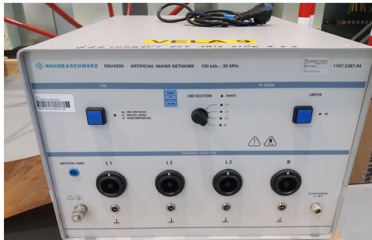
Figure 3: Line Impedance Stabilization Network (LISN) instrument used for the conducted emissions Rohde and Schwarz ENV4200, 150 kHz to 30 MHz, employing a transient limiter for the protection of the EMI receiver
