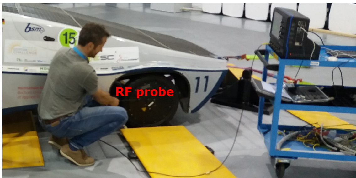
Figure 45: Near-field scan measurements of (a) the electric traction motor (integrated within the rim of the wheel) (b) vehicle's BUS module and (c) on-board driver's display, using RF probe and oscilloscope
