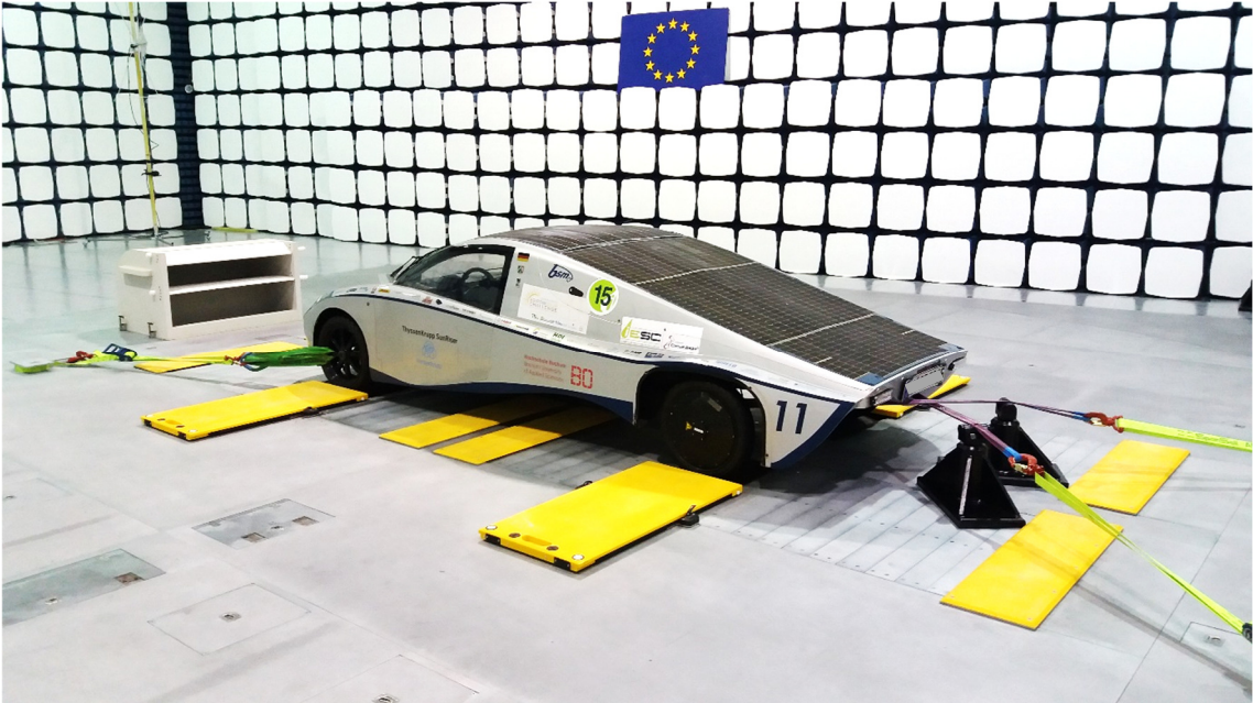
Figure 43: Solar car setup fixed with non-conductive straps on the roller bench inside VeLA 9 automotive EMC semi-anechoic chamber
