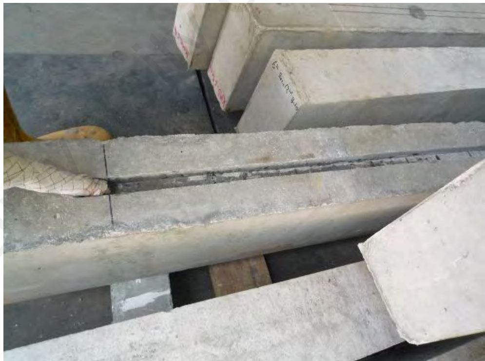
(c) Cleaning the groove with acetone
