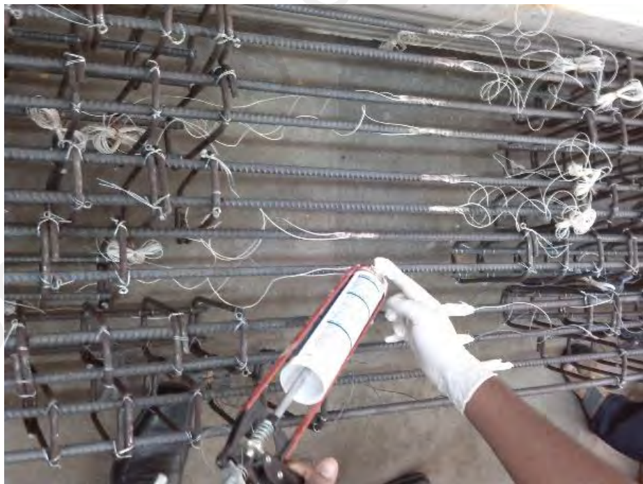
(b) Application of silicon on strain gauge Figure 3.5: Preparation and casting of RC beam
