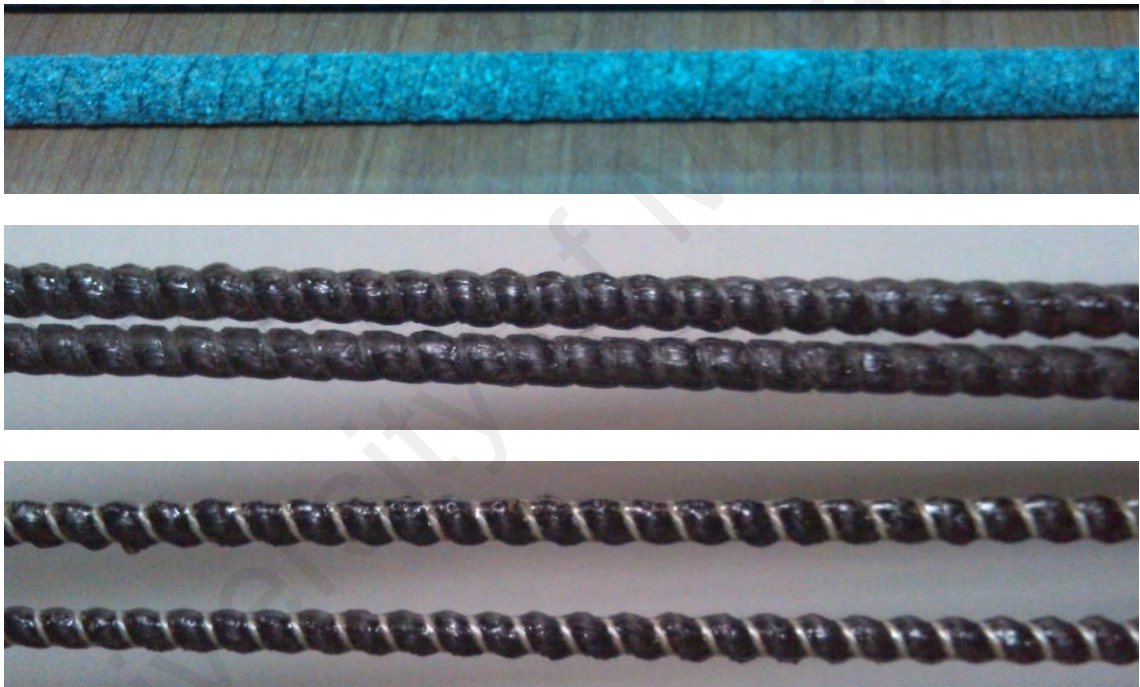
Figure 3.2: CFRP bar used for strengthening of RC beam
