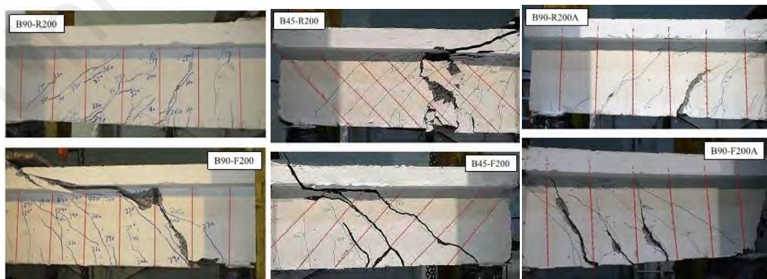
Figure 2.18: Failure modes of the strengthened beams(Rahal & Rumaih, 2011)
