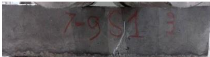
Figure 10. Cracking pattern at the failure of concrete with 1% of steel fiber.
