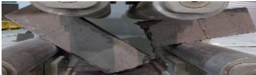
Figure 9. Cracking pattern at the failure of concrete with 0% of steel fiber.
