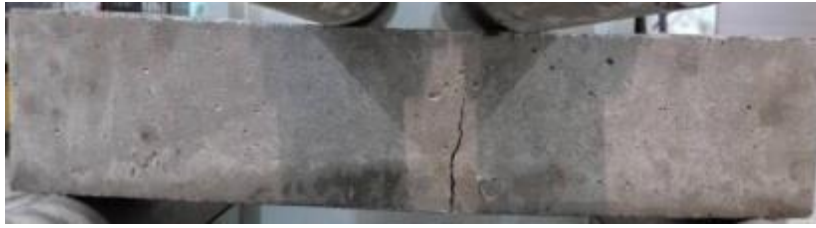
Figure 11. Cracking pattern at the failure of concrete with 2% of steel fiber.
