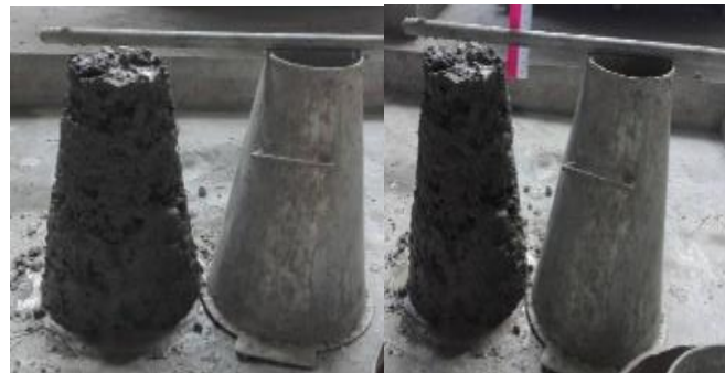
Figure 5. Concrete Slump Test
