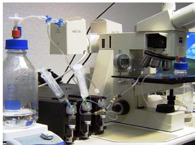
Image 3 experimental setup from left to right: distilled water in a reservoir on a hot plate, three pumps, tubes, manifolds, reflected-light microscope, connected microsystem, trash bin and PC in the background
