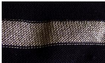
Figure 1 Textile electrodes consisting of electroconductive fibers integrated in knitted fabrics.
