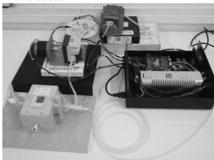
Figure 4: The experimental setup used for photoplethysmographic measurements consists of the tubing system placed in a wooden box and an infrared LED and phototransistor placed above them.
