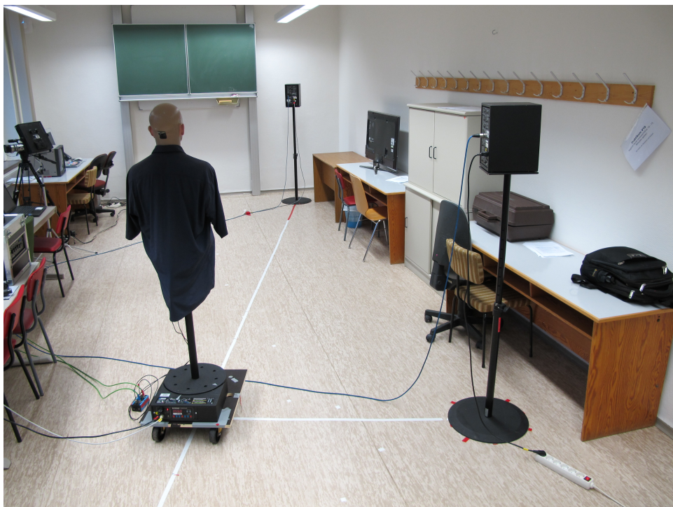
Fig. 7: Measurement setup in the seminar room with the loudspeakers turned by 180°.
