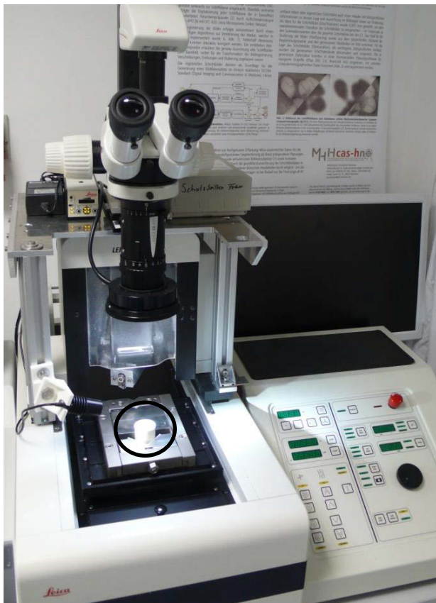
Figure 1: Automated microgrinding setup. Microscope with camera is mounted on top of the lifting head of the milling cutter. A sample (black circle) is clamped within the microtome. The control unit is shown on the right hand side of the microtome.
