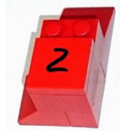
Figure 2: Artificial reference objects for determination of reconstruction accuracy of the automated microgrinding. Each sample was built from LEGO® bricks.
