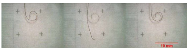
Figure 3: Recorded image of NiTi inlay before straightening at 5 °C, after straightening and at 45 °C after shape recovery (from left to right)
