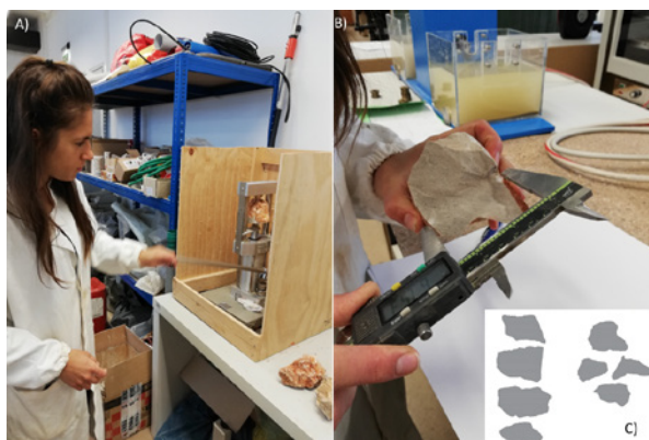
Figure 2. PLT device in the geotechnical laboratory at the University of Rijeka: a) load increase, b) determination of the average failure surface dimensions, c) digitalized exact failure surface
