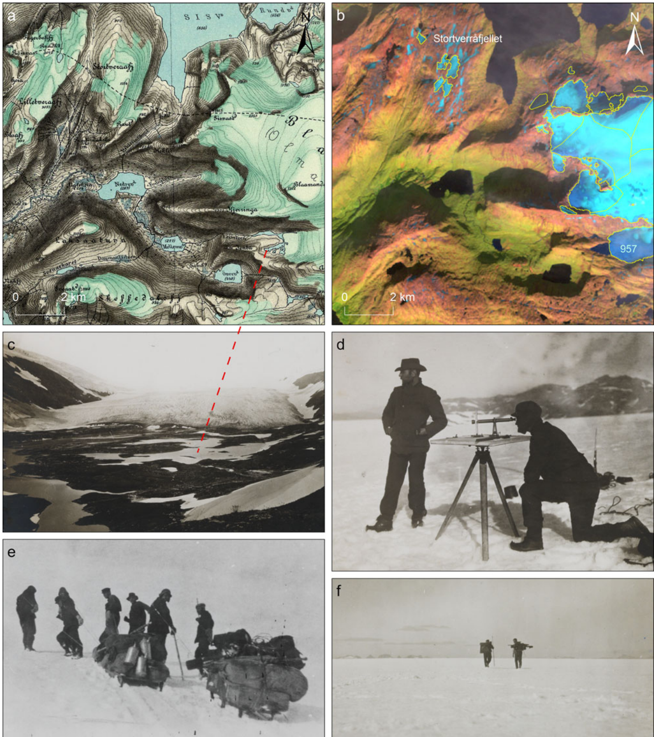
Fig. 3. (a) Section of map sheet L13 Saltaldalen (1 : 100 000; produced by T. Lundtvedt and O. Engh; published in 1910; Norges geografiske oppmåling; available from Kartverket) showing the western Blåmannsisen area at a scale of 1 : 150 000. (b) Landsat-7 scene from 7 September 1999 (bands 5, 4, 3) with the same extent as (a) (Paul and Andreassen, 2009). The 1999 glacier extent, as delineated by Paul and Andreassen (2009), is outlined in yellow. A substantial reduction in ice cover is apparent between the historical map and the satellite image, particularly on the mountain summits to the west of Blåmannsisen. (c) Historical survey photograph of Blåmannsisen's western outlet glacier with ID 957 (photo: Norges geografiske oppmåling, Nasjonalbiblioteket (National Library of Norway), SKM-S-L13-013). Note the proglacial meltwater system in front of the outlet that is mapped in some detail on the final L13 map. Dashed line shows location of the meltwater system in (a). (d) Plane tabling on top of Blåmannsisen (photo: Norges geografiske oppmåling, Nasjonalbiblioteket, SKM-S-L13-011). (e) Survey equipment is transported on sledges across Blåmannsisen (photo: Norges geografiske oppmåling, Nasjonalbiblioteket, SKM-S-L13-028). (f) Surveyors crossing Stortverråfjellet (photo: Norges geografiske oppmåling, Nasjonalbiblioteket, SKM-S-L13-010). All photographs were taken during the original field surveys.
