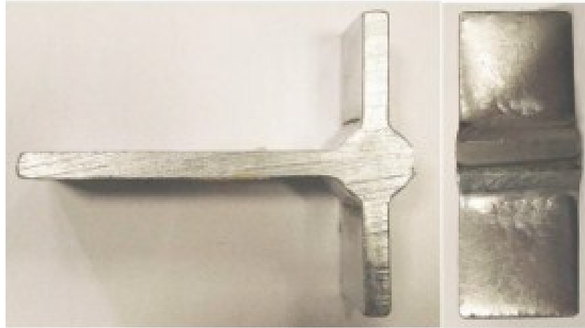
Fig. 12. Typical broken specimens under fatigue test [39].
