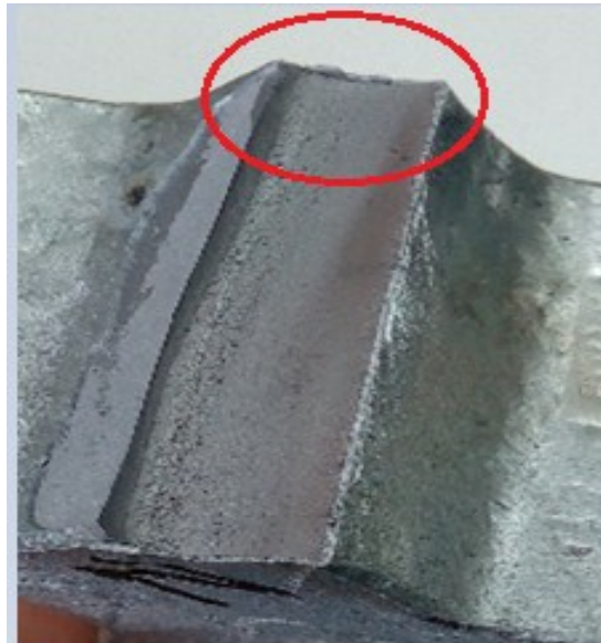
Fig. 18. Specimen No. 5, macro observation of fracture surface after cyclic loading.
