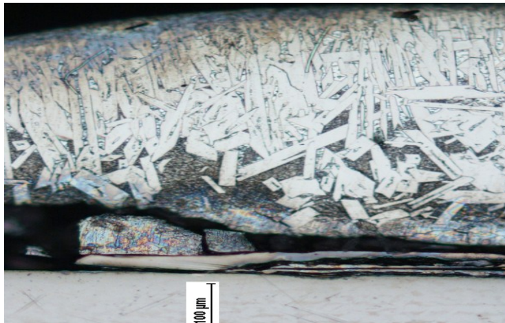
Fig. 19. Debonding between the base material and coating.
