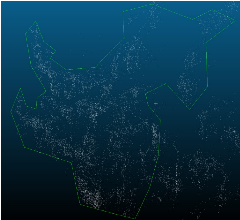
Figure 36: Extraction of the crown intensity data using the cutting tool.
