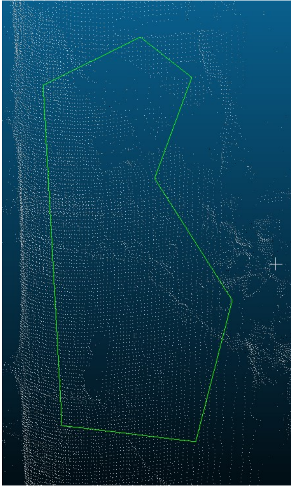
Figure 35: Extraction of the stem intensity data using the cutting tool.
