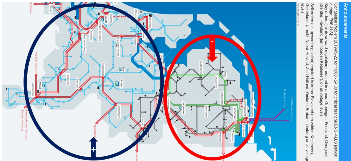
Figure 16: A congestion announcement on 22.9.2019 from 7 pm to 12 am for Ketelmeer area. Adapted from (GOPACS 2019b; TenneT 2019).
