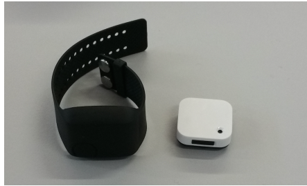
Figure 6.2. Empatica E4 biophysical sensor (left) and Narrative Clip Wearable Camera (right)
