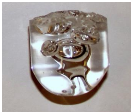
Figure 6.19 - First solid and clear PMMA sample. High amount of gas bubbles is visible.
