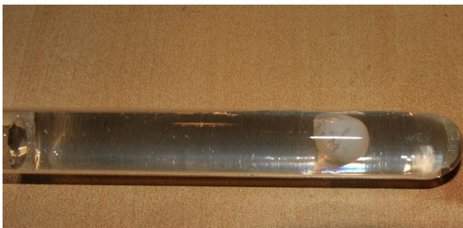
Figure 6.17 - Excess initiator in the air bubble.
