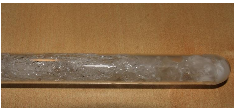
Figure 6.18 - Result of the too fast and too exothermic polymerization.
