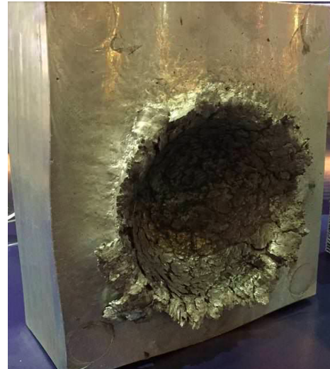
(b) Consequences of the impact of a 15 g piece of plastic on a block of aluminium at about 24 000 km/h.
