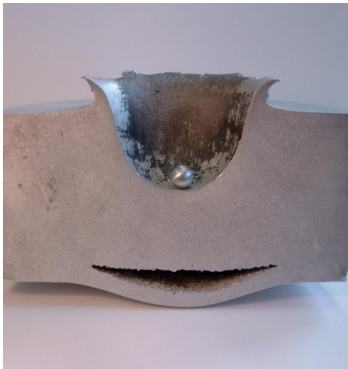
(a) Hypervelocity impact study example. A 1.2 cm diameter aluminium sphere impact at 6.8 km/s on a 18 cm thick block of aluminium.[18].
