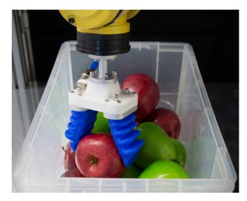
Figure 2.13: Example of a soft gripper [25].
