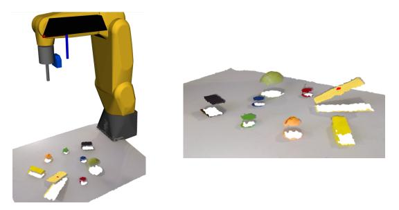
Figure 6.11: Representation, with a red dot, of the centroid of the object to grab in relation to the Kinect's frame.
