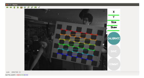
Figure 4.9: Calibration window with the highlighted checkerboard.
