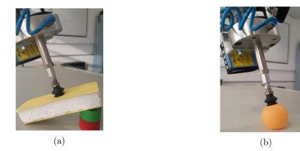
Figure 6.17: Gripper properly positioned to grasp different objects, one a flat surfaced object, (a), and the other a curved object, (b).
