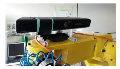
Figure 4.10: Kinect with the IR projector blocked for the intrinsic calibration of the IR (depth) camera.
