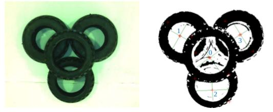
(a) Image captured by the monocular camera. (b) Detection of 4 candidate objects.
