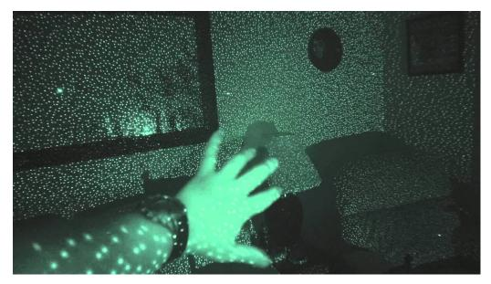
Figure 3.4: The laser grid used by the Kinect to calculate depth.
