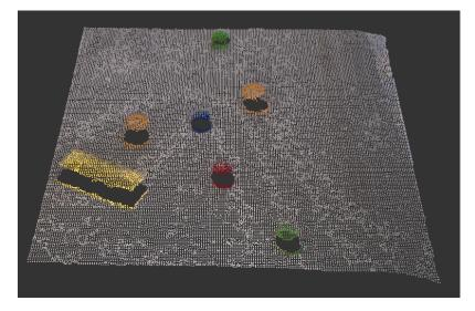
Figure 5.4: Point cloud after the VoxelGrid filter.
