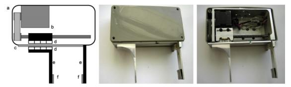
Figure 2.11: Gripper with force feedback for handling different types of fruits and vegetables [23].
