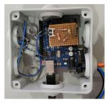
Figure 7.5: Box with the Arduino and all the connections properly stored.
