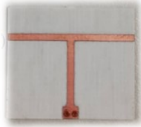
Figure 3.9: Short stub circuit.
