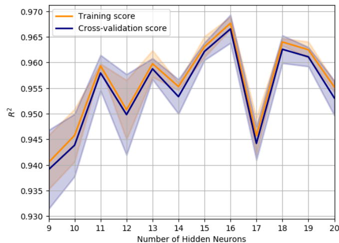
Figure 3.21: Validation curve of trained ANN-model with a range of hidden neurons from nine to twenty for one hidden layer.
