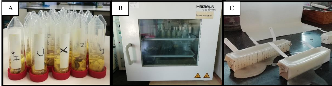
Fig. 8 A: Mussels in ethanol 70%; B: Vacuum stove with the samples embedded in paraffin; C: Paper molds with samples and paraffin.
