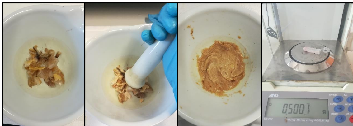
Fig. 5 Homogenization of mussel's frozen tissue with liquid nitrogen.
